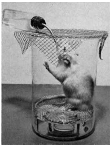
Fig. 2.—Assembled metabolism cage containing a rat.
